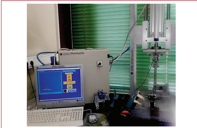
Figure 4. The experimental device "PROCRUSTIS" was used for the pull-out experiments.
